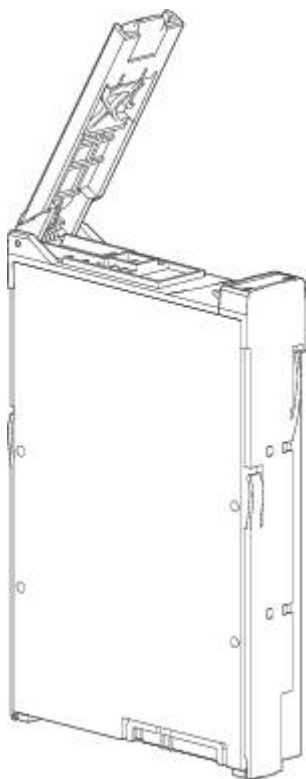
Figure 71. LFF drive carrier module in open position
